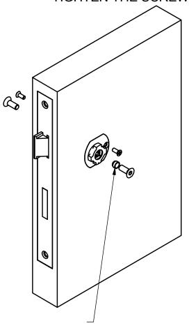
we advise to use conical spacers to expand the spindle
